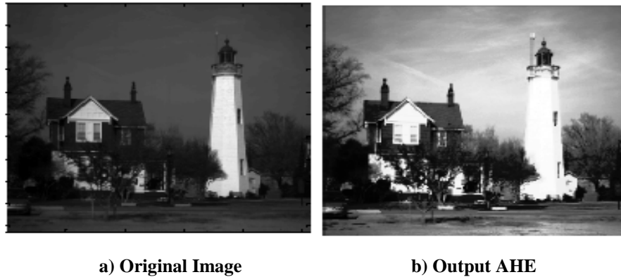
Figure 2: The Results of Adaptive Histogram Equalization (a) Original Image (b) Output Results of Adaptive Histogram Equalization
